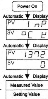
First, press (SET) key to make the SV display in the flashing state. Then press (<R/S) key to find the place number of required setting temperature. Third, press (V) or (Λ) key to set the required temperature. After ending of the setting, press (SET) key again to be SV/PV normal display state.
